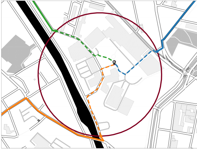
Figure 3: The intuition behind our attack: we search the protected location (shown as a black marker) as the point where the theoretical paths (based on reported distances, shown by dashed lines) starting from the EPZ entry gates (in different directions, shown by different colors) intersect.
