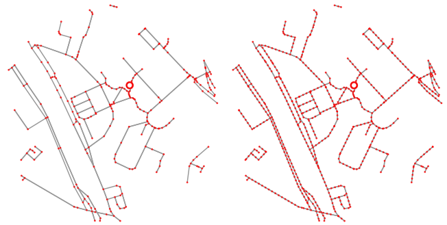
(a) Example road network graph G for one EPZ. (b) Road network with node resolution increased through chaining.
